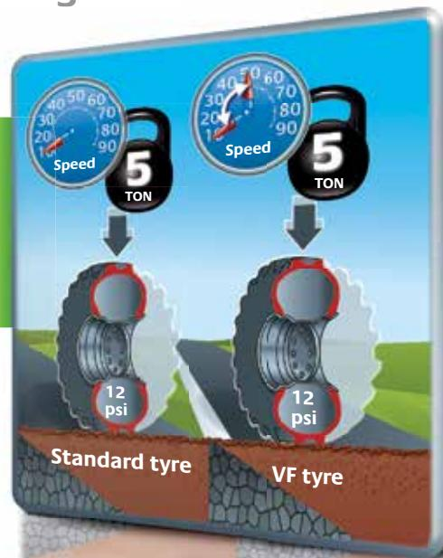
You should never exceed either the recommendations from the vehicle manufacturer or the legal maximums for axle load or speed.
